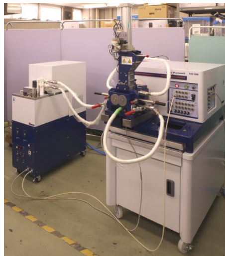
(Banbury blades type mixer model BR250 with oil circulation bath Note: Shown base unit is old generation model)
